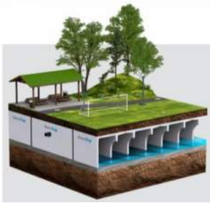
Figure 2: typical Infiltration Gallery (Source: StormTrap)
