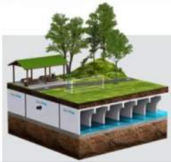
Figure 2: Typical Infiltration Gallery (Source: StormTrap)
