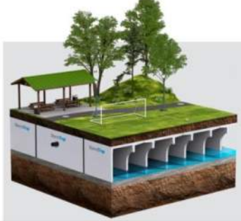
Figure 2: Typical Infiltration Gallery (Source: StormTrap)
