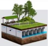
Figure 2: Typical Infiltration Gallery (Source: StormTrap)
