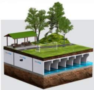
Figure 2: typical Infiltration Gallery (Source: StormTrap)
