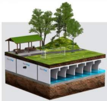
Figure 2: typical Infiltration Gallery (Source: StormTrap)
