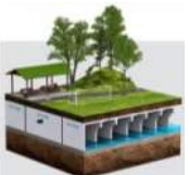
Figure 2: Typical Infiltration Gallery (Source: StormTrap)
