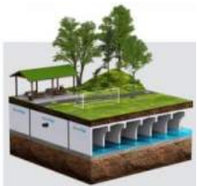
Figure 2: Typical Infiltration Gallery (Source: StormTrap)
