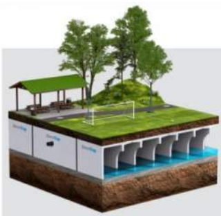
Figure 2: typical Infiltration Gallery (Source: StormTrap)
