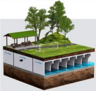
Figure 2: typical Infiltration Gallery (Source: StormTrap)
